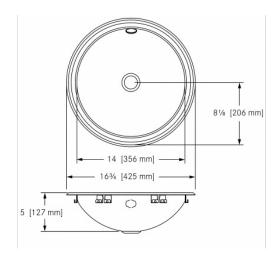
Single compartment self rimming vanity basin less faucet ledge. 18 gauge (1.2 mm), type 304 (CNS 18/10) stainless steel. Mrror finished rim, #4 satin finished bowl. Undercoated to reduce condensation and resonance. Includes factory applied rim seal, cutout template, and installation hardware. Certified to ASME A112.19.3-2008 / CSA B45.4-08.
