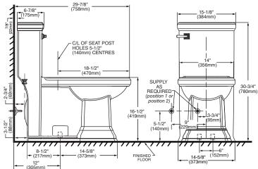
IMPORTANT: Water supply on the wall is required at 3-3/4" (95mm) or 9" (229mm) from centreline of the toilet (see rough-in). First suggested position is hidden behind the toilet. The geometry of the toilet gives space for this installation. The second suggested position is next to the toilet. Between these two positions, the space for the supply between wall and toilet is limited to 3-1/4" (83mm). In this case, check your supply and hose dimensions.
