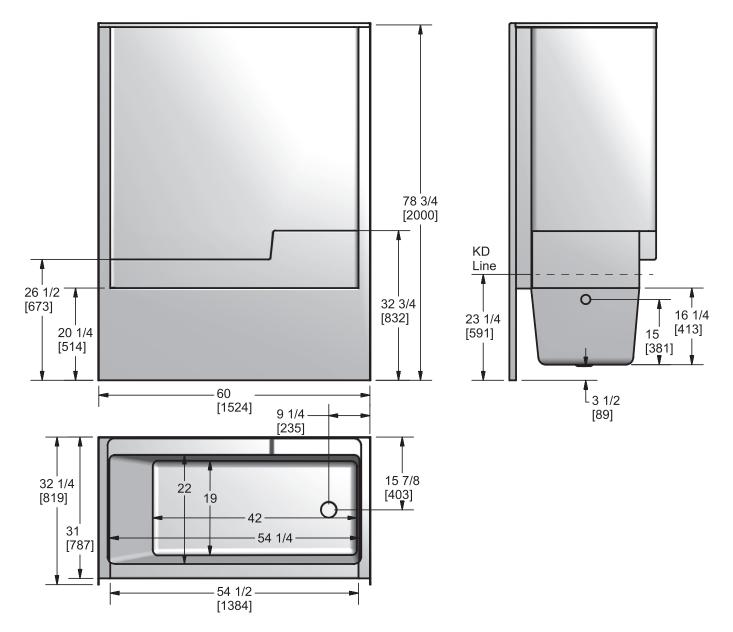
Measurement tolerances ± 1/4" (6.3 mm)
