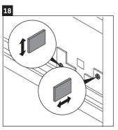
Level the vanity drawer by adjusting the two screws.
