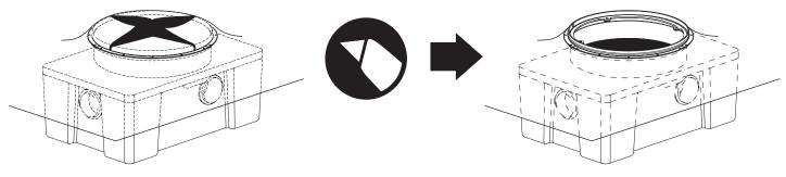
Cut and remove membrane from the accessway of the FCR1
