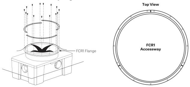
Using the self tapping screws provided, fasten the (3) Clamping Bars directly to the flange of the FCR1
