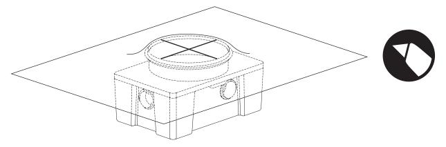
Cut a relief " + " pattern in the membrane directly over the opening of the FCR1 accessway.
