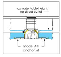
At risk areas include but are not limited to tidal surge areas, floodplains and areas that receive storm water. Billy Goat™ models that are direct buried in high water table scenarios must be installed with an anchor kit. Model SI-50 uses model AKI anchor kit.
