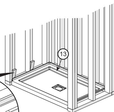
With a 1/8" bit, drill holes in the fastening flange then secure the base to all the wall studs with #8 x 1 1/4" screws (not included). **Only pre-drill the flange not the studs.**
