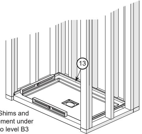
If needed, use wood shims between the studs and the fastening flange to maintain centered position of base.
