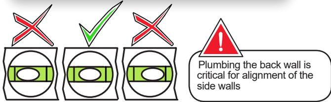
**Quick tip** Installing the walls temporarily will ensure proper wall alignment before permanent installation. Make sure the wall is plumb and centered on the base.
