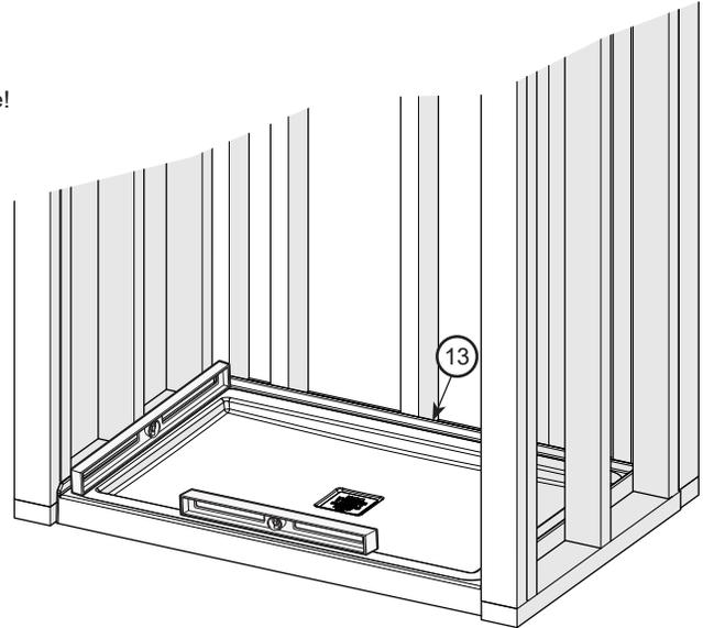
Lift the base. Insert wood shims on the floor around the outline of the base on the previously marked spots to compensate leveling.
