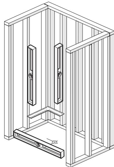
Cut out an approximate 6" x 6" opening around the drain center outlined by measurements C and D. See image to the right and the chart above. We recommend that a plumber completes the drain pipe connection.
