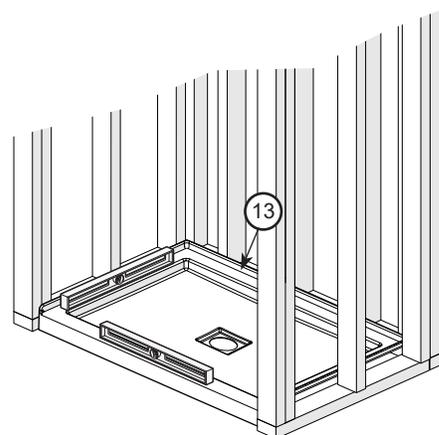
If needed, use wood shims between the studs and the fastening flange to maintain centered position of base.
