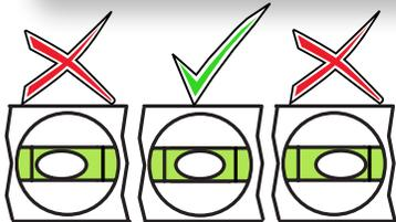
Leveling the floor is critical for a properly aligned installation. Auto leveling cement can be used to level floor. Be careful not to block the drain hole position.
