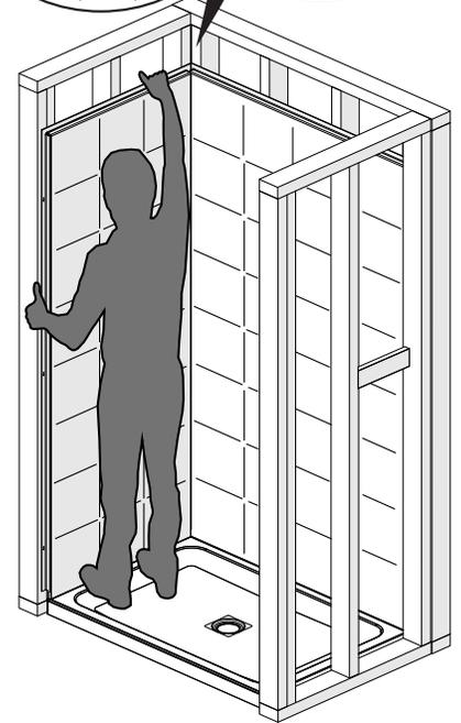
Install the side wall (15) with the faucet hole. Lift the wall approximately 3 inches above the threshold of the base, push it completely against the back wall then slide the side wall into position.
