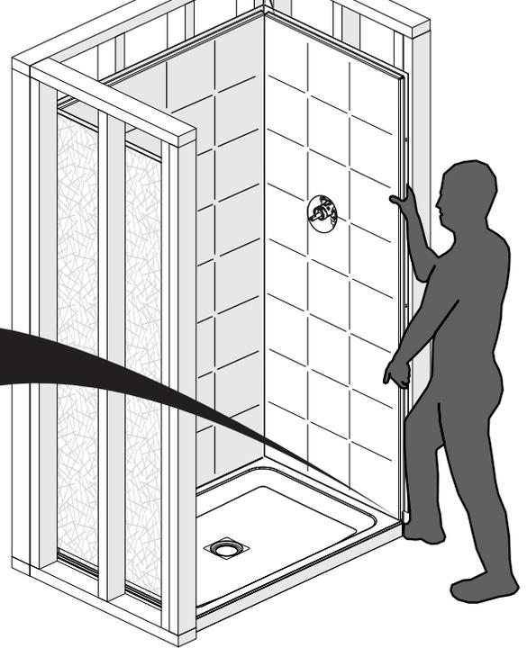
With a 1/8" bit, drill holes in the side wall fastening flange (15) at the top aligned with each stud. Only pre-drill the flange not the studs. Then, secure the side wall (15) with one #8 x 1 1/4" screw (not included) in one of the pre-drilled holes.
