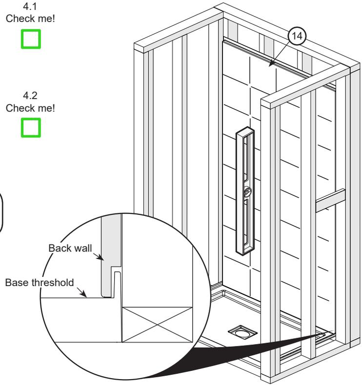
With a 1/8" bit, drill holes in the back wall fastening flange (14) at the top aligned with each stud. **Only pre-drill the flange not the studs.** Then, secure the back wall (14) with **one #8 x 1 3/4"** screw (not included) in one of the pre-drilled holes.
