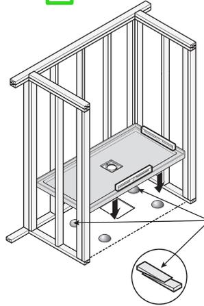
Shims and cement under to level B3 bases
