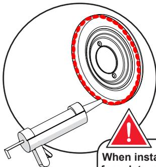
**When installing the faucet faceplate or other components, be sure to silicone the outer edge.**
