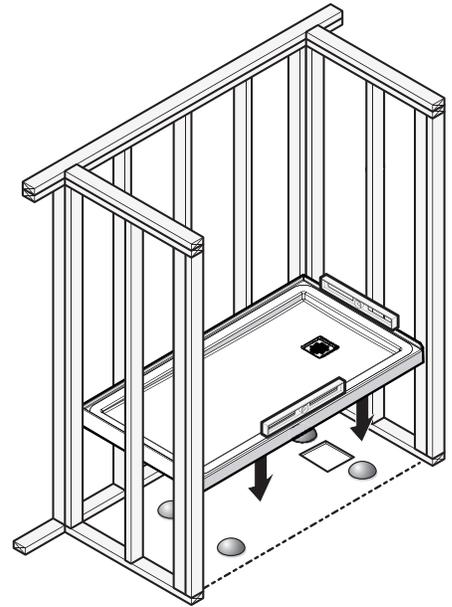
If needed use wood shims between the studs and the fastening flange to maintain centered position of base.
