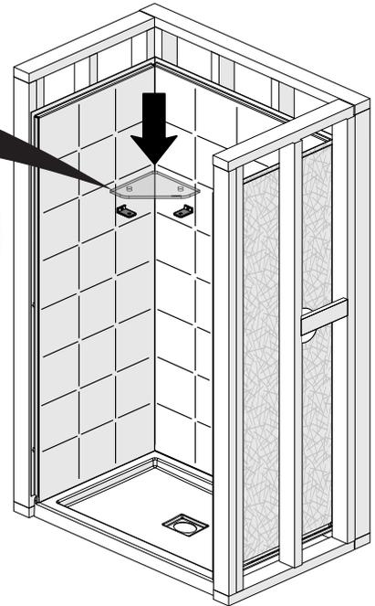
Insert the washers (8) in the shelf support cap (9). Align and insert the shelf support caps (9) with the holes of the glass and the holes of the shelf brackets (6). Screw from the bottom of the shelf with the # 10 x 1/2" screws (10) and tighten by hand with the Allen key (11).
