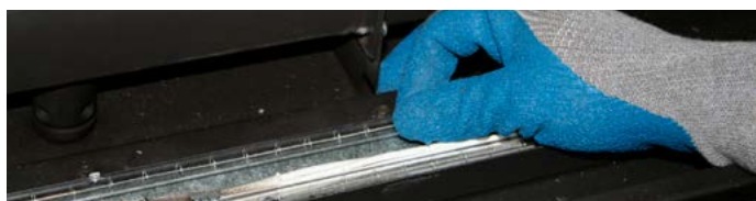
Figure 29.c Rotate newly replaced bulbs in a full circle. Place glass cover back in the burner tray.
