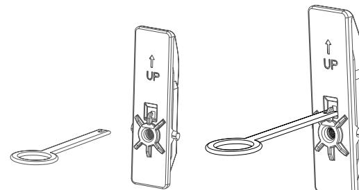
**6** With pull tab up, insert the anchor all the way into the hole in the wall.
