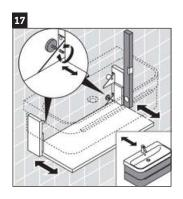
Check the vanity is leveled and make adjustments using screws.
