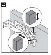
Check the screws which allow adjustment of the unit. The top screw will adjust up and down, and the bottom screw will adjust front and back.
