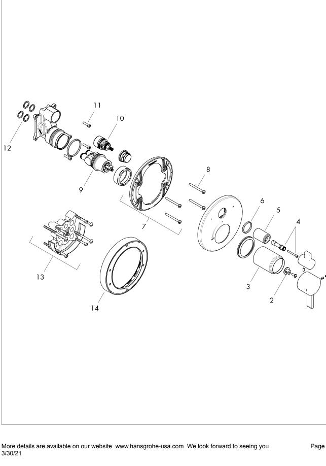
Ecostat Pressure Balance Trim S with Diverter Finishes : brushed nickel Part no. : 04447820
