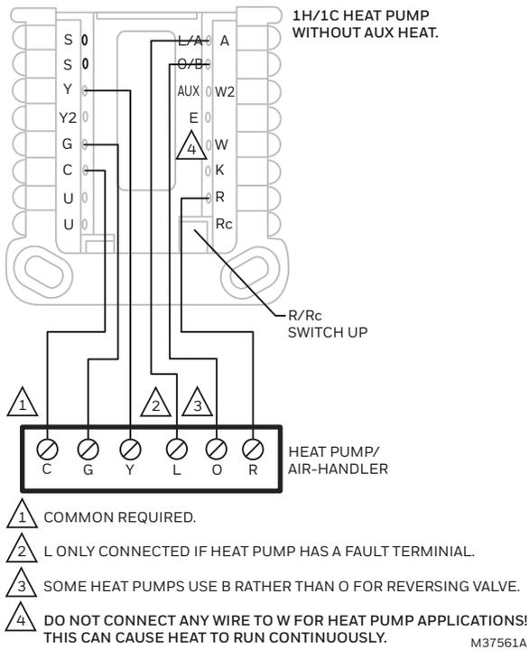
Fig. 22. 1H/1C heat pump without aux heat.
