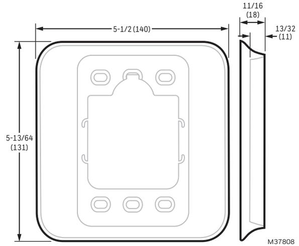
**Fig. 5. Dimensions of cover plate in in, (mm)**
