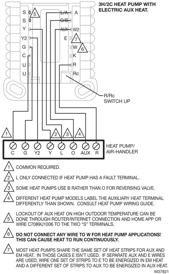
Fig. 25. 3H/2C heat pump with electric aux heat.
