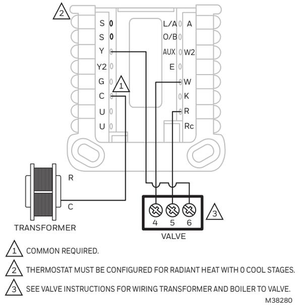
**Fig. 20. Series 20 valve (power open and power closed).**
