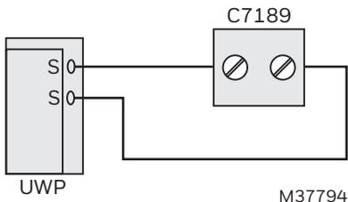
**Fig. 38. Wiring 1 C7189 sensor.**
