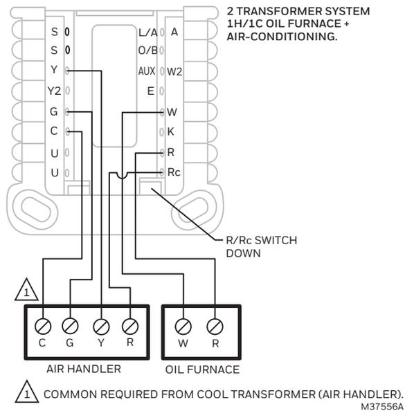
**Fig. 16. 2 Transformer system; 1H/1C oil furnace.**
