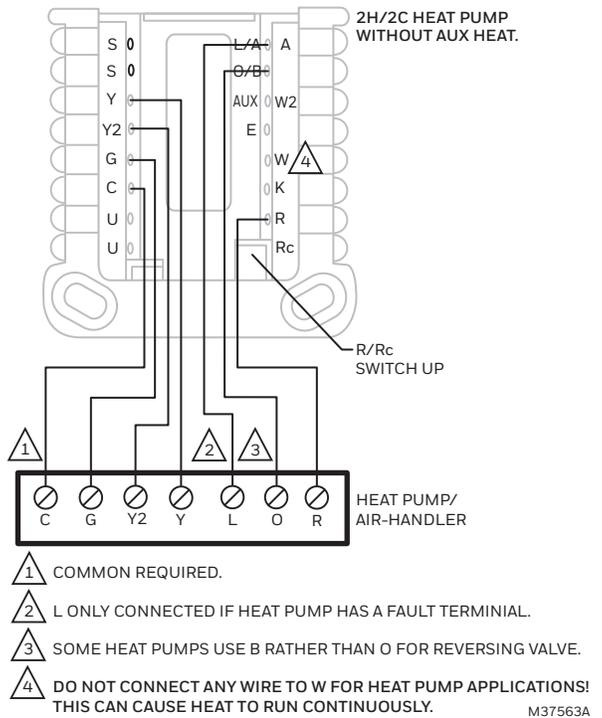
Fig. 24. 2H/2C heat pump without aux heat.
