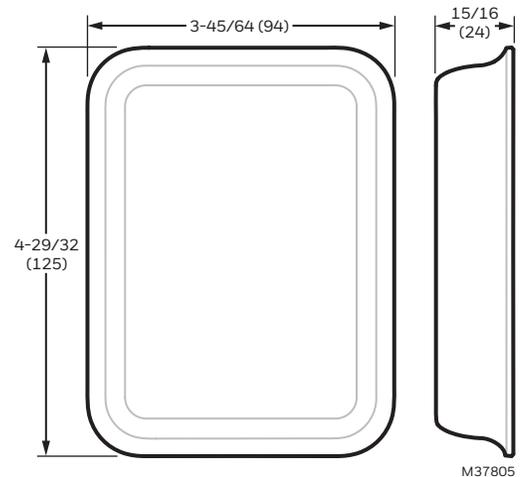
**Fig. 2. Dimensions of thermostat in In. (mm).**
