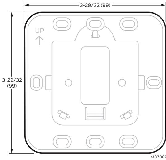
**Fig. 4. Dimensions of J-Box Adaptor in In. (mm).**
