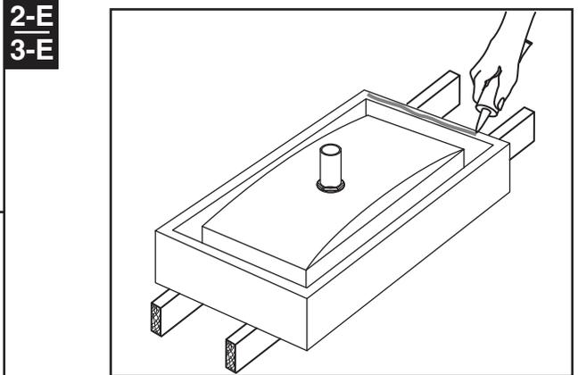
After checking fit and alignment, turn sink upside down and apply a generous portion of silicone adhesive around the under side of the rim near the edge. Place sink in position. Wipe off excess adhesive.
