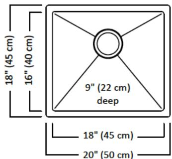
Material Construction 18 gauge, 18-10 stainless steel, type 304
