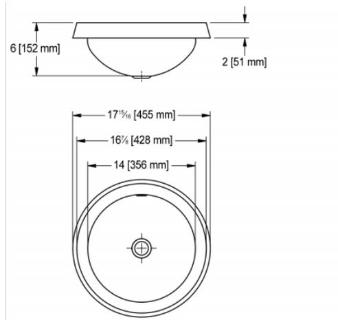
Single compartment semi-recessed vanity basin less faucet ledge. 18 gauge (1.2 mm), type 304 (CNS 18/10) stainless steel. Mirror finished rim, #4 satin finished bowl. Undercoated to reduce condensation and resonance. Includes cutout template and installation hardware. Certified to ASME A112.19.3-2008 / CSAB45.4-08.
