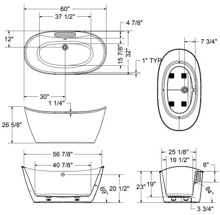
( : Recommended faucet area of 15" (L) x 3-1/2" (W). Depth recommended for straight pipes 8".
