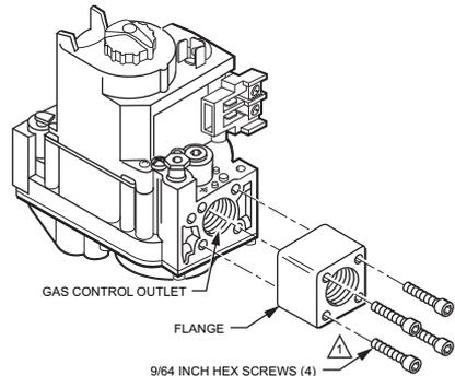
⚠️ DO NOT OVERTIGHTEN SCREWS. TIGHTEN TO 25 INCH-POUNDS.
