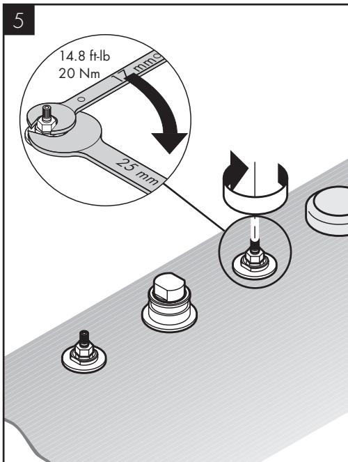
Tighten the new cartridges.
