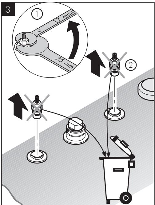
Remove the cartridges.
