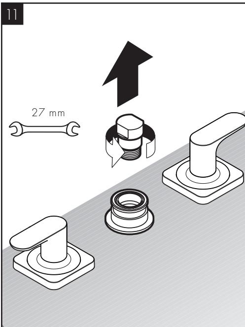
Remove the plug from the diverter housing.
