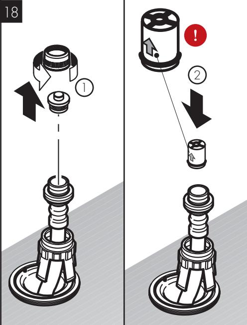
Remove the brass plug and nut from the high pressure hose.
