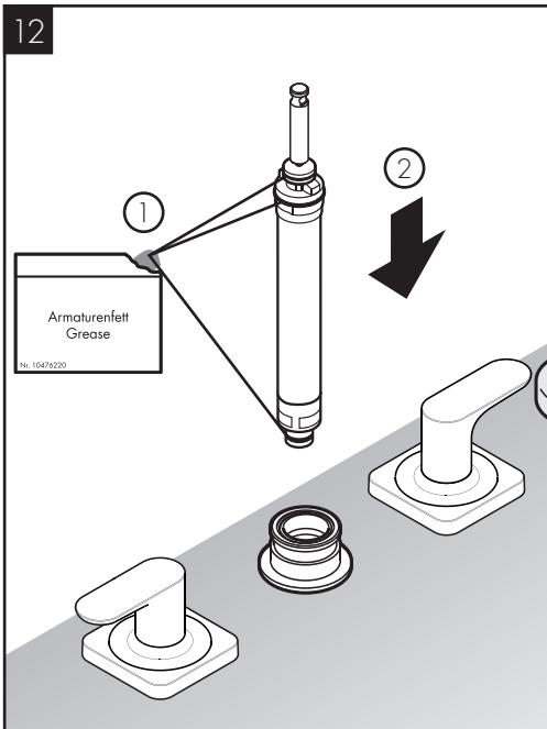
Lightly lubricate the o-rings on the diverter using white plumbers grease.
