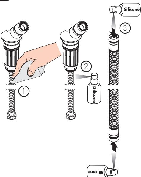
Lubricate the handshower hose using silicone spray.
