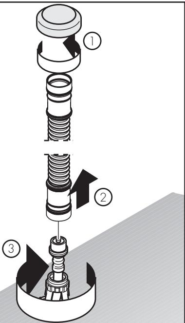
Remove the plaster shield from the Secuflex hose.
