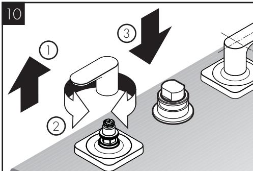
If it is not correct, remove, rotate, and reinstall the handle.
