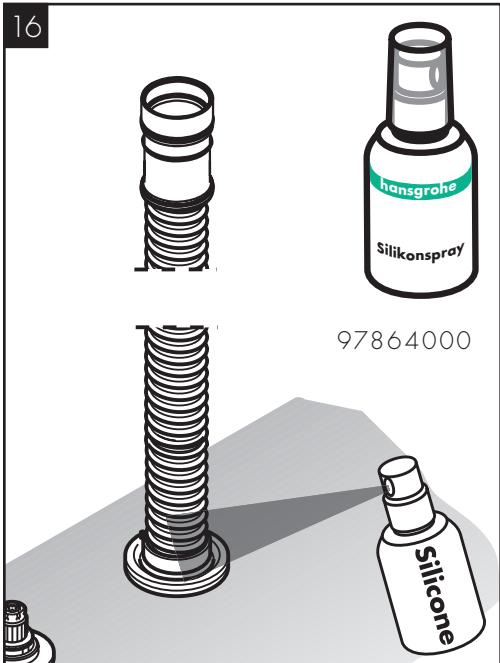
Lubricate the Secuflex hose using silicone spray.
