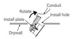
(3) The install plates will position themselves onto the drywall.
