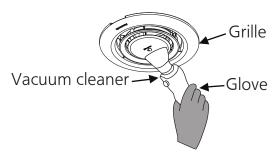
Using a cloth dampened with kitchen detergent, remove any dirt from the grille body. Wipe dry with a clean cloth.
