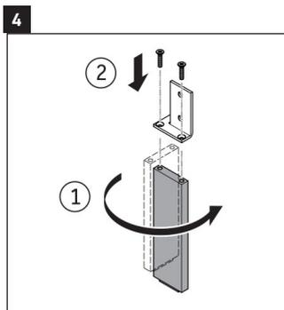
4 Turn leg counter-clockwise and screw two screws in.
