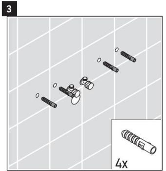
3 The plastic anchors provided are for concrete wall applications.
