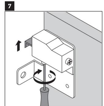
7 Using a screwdriver, adjust the vanity mounting hinge system clockwise.
