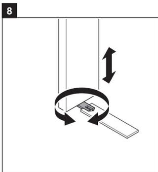
Using supplied key, adjust the legs height.
