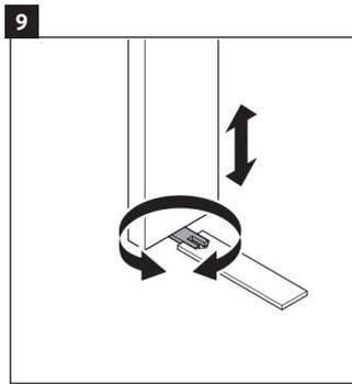
Using supplied key, adjust the legs height.
