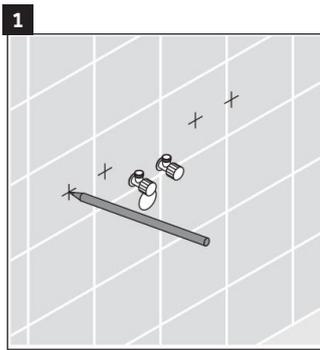
1 Reference the vanity specification to establish the position of mounting bolts, mark the holes to be drilled for the anchors.
