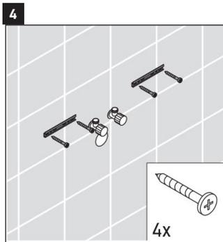
4 For wood stud walls, bolts should be screwed into wood backing.
