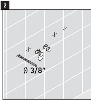
2 Using a 3/8" drilling bit, drill the anchor holes that have been marked.
