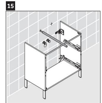
Reference the washbasin specification to establish the position of mounting bolts, mark the holes to be drilled for the anchors.
