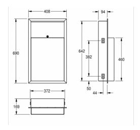
Waste bin for recessed mounting, stainless steel, surface satin finished, material thickness 22 gauge rounded edges, cylinder lock with Franke standard key, mounting with in-wall frame, including stainless steel screws and dowels.
