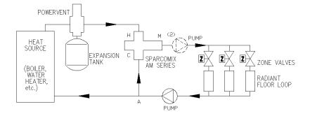
CAUTION: DO NOT INSTALL PUMP BETWEEN CONNECTION "A" AND HEAT SOURCE. The installation of the pump at this point would result in NO FLOW through the radiation loop(s).
