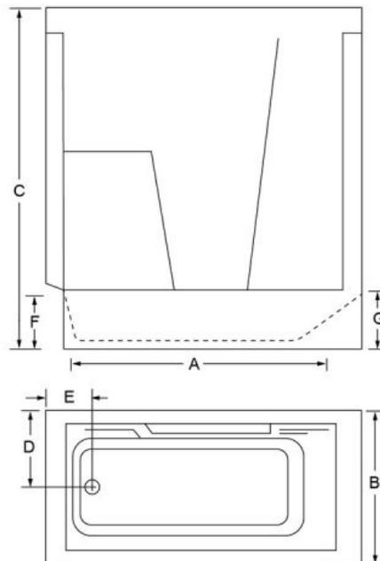
Product is made of Gel-coat surface & reinforced with heavy-duty fiberglass. The unit has a 1" nailing flange on front & top edges (except for drop in tubs). Product measurements are to the outside of nailing flange. Measurements are plus (+) or minus (-) 1/4".
