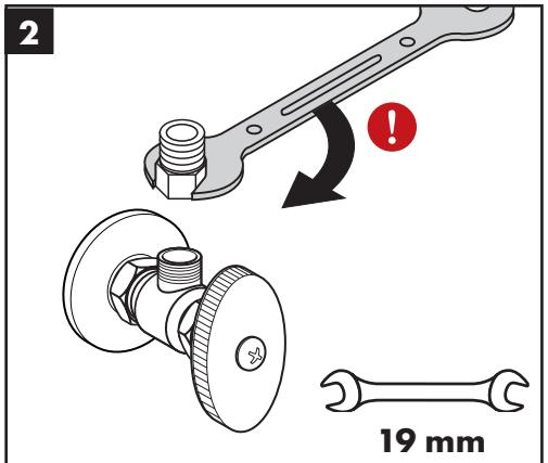
Install the adapters on the stops.
