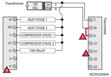
Typical wiring of a 3-heat / 2-cool heat pump system with two transformers (example - oil forced air backup heat)
