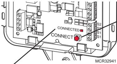
Press and release the **CONNECT** button at the EIM or Wireless Adapter, and make sure the "Connected" light is flashing green.
