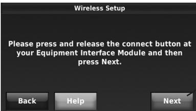
While the EIM light is flashing, press **NEXT** to link the thermostat with the EIM. After a brief delay, the screen will display "Device Connected."
