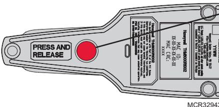
Press and release the button on the bottom of the Internet Gateway. After a short delay, the RedLINK status light will glow steady green.
