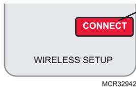
Press **CONNECT** on the Portable Comfort Control display screen. Press **DONE** when the screen displays "Connected," then exit or continue to link another thermostat.
