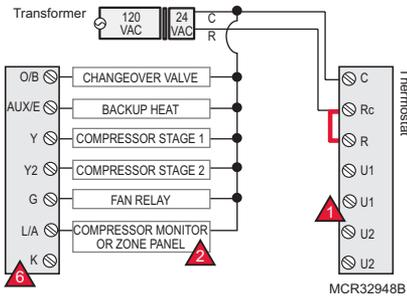
Typical wiring of a 2-heat / 2-cool conventional system with one transformer
