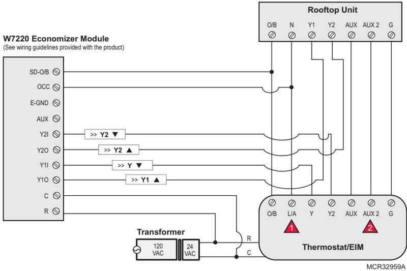
Typical wiring of a W7220 Economizer Module for a conventional system, using a Prestige THX9321 thermostat or Equipment Interface Module.
