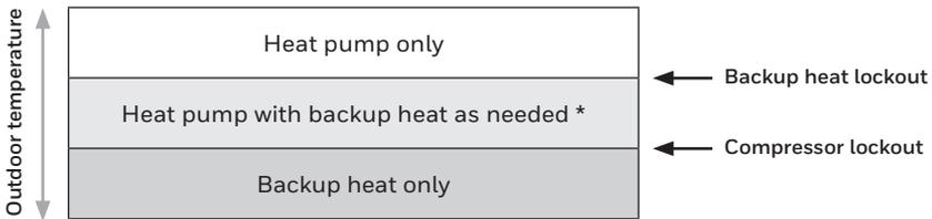
\* No backup heat unless indoor temperature drops to selected Backup Heat Differential setting, or Backup Heat Upstage Timer expires. Heat pump stays ON when backup heat turns on.
