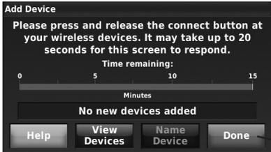
While the Add Device screen is displayed on the thermostat, press and release the **CONNECT** button on each wireless device, as described below. Accessories need to be at least 2 feet away from the thermostat or EIM during the linking process.
