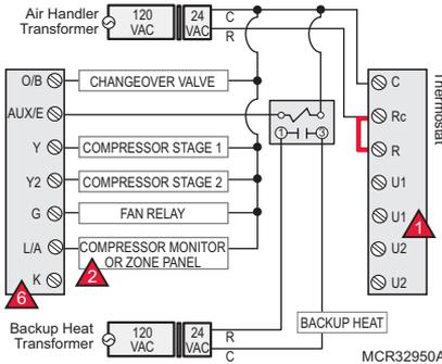
Typical wiring for geothermal radiant heat, geothermal forced-air and backup heat with one transformer. See page 19 for operation.
