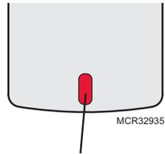
If the status light turns red, the sensor did not link with the thermostat.
