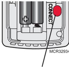
Press and release **CONNECT**. After a short delay, the status light will glow green for 15 seconds.
