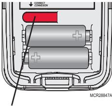
Press and release **CONNECT**. After a short delay the thermostat will display "Wireless Outdoor Sensor added" on the Add Device screen.
