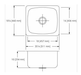
Single compartment undermount sink. 18 gauge (1.2 mm), type 316 (EN1.4401 17/12/2) stainless steel. Exposed surfaces are #4 satin finished. Undercoated to reduce condensation and resonance. Includes waste fitting, cutout template, and Universal Installation System hardware. Certified to ASME A112.19.3-2008 / CSA B45.4-08.
