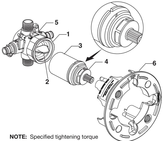
**NOTE:** Specified tightening torque of **BONNET NUT (1)** is critical to assure sealing function.
