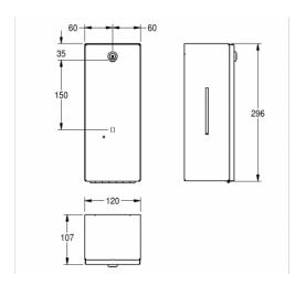
Touch free soap dispenser for wall mounting, stainless steel, surface satin finished, material thickness 20 gauge folded front cover, cylinder lock with Franke standard key, infrared sensor activity for non-touch operation, LED-light shows battery status. Needs 4 pieces 1.5 V (=9 V) alkaline AA batteries. Suitable for liquid soaps and lotions, 800 ml soap tank, depending on soap between 0.6 and 1.1 ml is dispensed, including stainless steel screws and dowels.
