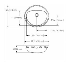
Single compartment self rimming vanity basin with faucet ledge. 18 gauge (1.2 mm), type 304 (CNS 18/10) stainless steel. Mirror finished rim, #4 satin finished bowl. Undercoated to reduce condensation and resonance. Includes factory applied rim seal, cutout template, and installation hardware. Certified to ASME A112.19.3-2008 / CSA B45.4-08.
