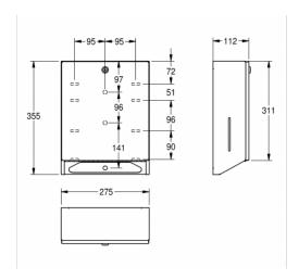
Paper towel dispenser for wall mounting, stainless steel, surface satin finished, material thickness 22 gauge, folded front cover, cylinder lock with Franke standard key, inspection windows on sides, loading capacity 500 - 800 pcs. of paper depending on convolution, including stainless steel screws and dowels.
