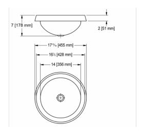
Single compartment semi-recessed vanity basin less faucet ledge. 18 gauge (1.2 mm), type 304 (CNS 18/10) stainless steel. Mirror finished rim, #4 satin finished bowl. Undercoated to reduce condensation and resonance. Includes cutout template and installation hardware. Certified to ASME A112.19.3-2008 / CSA B45.4-08.
