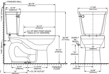
NOTES: THIS TOILET IS DESIGNED TO ROUGH-IN AT A MINIMUM DIMENSION OF 356MM (14") FROM FINISHED WALL TO C/L OF OUTLET. SUPPLY NOT INCLUDED WITH FIXTURE AND MUST BE ORDERED SEPARATELY.
