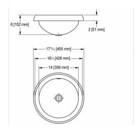
Single compartment semi-recessed vanity basin less faucet ledge. 18 gauge (1.2 mm), type 304 (CNS 18/10) stainless steel. Mirror finished rim, #4 satin finished bowl. Undercoated to reduce condensation and resonance. Includes cutout template and installation hardware. Certified to ASME A112.19.3-2008 / CSA R45 4-08
