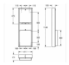
Paper towel dispenser, waste bin combination for wall mounting, stainless steel, surface satin finished, material thickness 22 gauge folded front cover, cylinder lock with Franke standard key, loading capacity 500 - 800 pcs. of paper depending on convolution, waste bin with approx 23 litre capacity, including stainless steel screws and dowels.
