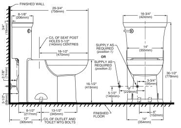
IMPORTANT: Water supply on the wall is required at 3-3/4" (95mm) or 9" (229mm) from centreline of the toilet (see rough-in). First suggested position is hidden behind the toilet. The geometry of the toilet gives space for this installation. The second suggested position is next to the toilet. Between these two positions, the space for the supply between wall and toilet is limited to 3-1/4" (83mm). In this case, check your supply and hose dimensions.
