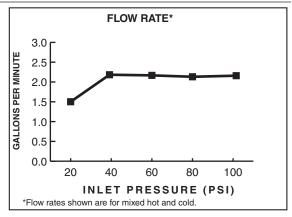
2.2 gpm/8.3 L/min. FLOW RATE
