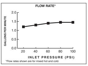
1.5 gpm/5.7 L/min. FLOW RATE
