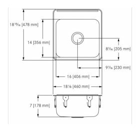
Single compartment self rimming drop-in sink with faucet ledge. 20 gauge (0.9 mm), type 302 (CNS 18/8) stainless steel. Exposed surfaces are #4 satin finished. Undercoated to reduce condensation and resonance. Includes waste fitting, factory applied rim seal, cutout template, and factory installed EZ TORQUE™ fasteners. Certified to ASME A112.19.3-2008 / CSA B45.4-08.
