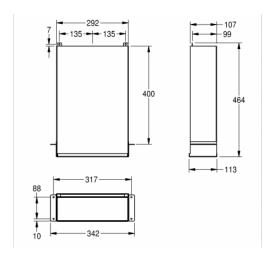
Paper towel dispenser for hidden mounting behind wall and mirror, stainless steel, surface satin finished, material thickness 22 gauge for 600 - 800 paper towels, depending on convolution, filling from bottom, including stainless steel screws and dowels.
