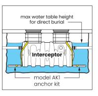
areas, floodplains and areas that receive storm water. Billy Goat™ models that are direct buried in high water table scenarios must be installed with an anchor kit. Model SI-250 uses model AKI anchor kit.
