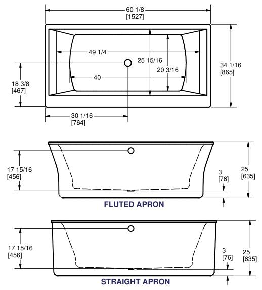
Measurement tolerances ± 1/4" (6.3mm)
