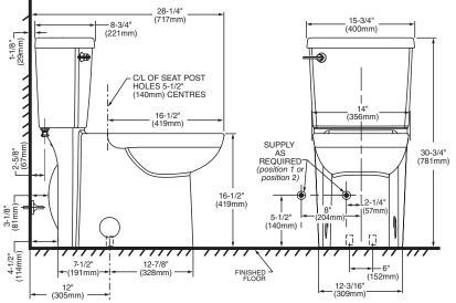
IMPORTANT: Water supply on the wall is required at 2-1/4" (57mm) or 8" (204mm) from centreline of the toilet (see rough-in). First suggested position is hidden behind the toilet. The geometry of the toilet gives space for this installation. The second suggested position is next to the toilet. Between these two positions, the space for the supply between wall and toilet is limited to 4-1/2" (114mm). In this case, check your supply and hose dimensions.
