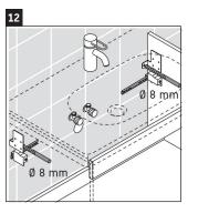
Using the appropriate bit for the wall material, drill pilot holes.
