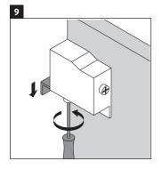
Using a crewdriver adjust the vanity mounting hinge system counter-clockwise.
