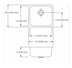
Single compartment undermount sink. 18 gauge (1.2 mm), type 304 (CNS 18/10) stainless steel. Exposed surfaces are #4 satin finished. Undercoated to reduce condensation and resonance. Includes waste fitting, cutout template, and installation hardware. Certified to ASME A112.19.3-2008 / CSA B45.4-08. Center back waste location, 3 1/2" (89 mm) crumb cup strainer with 1 1/2" (DN38) brass tailpiece.
