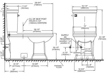
IMPORTANT: Water supply on the wall is required at 2-1/4" (57mm) or 8" (204mm) from centreline of the toilet (see rough-in). First suggested position is hidden behind the toilet. The geometry of the toilet gives space for this installation. The second suggested position is next to the toilet. Between these two positions, the space for the supply between wall and toilet is limited to 3-1/2" (88mm). In this case, check your supply and hose dimensions.
