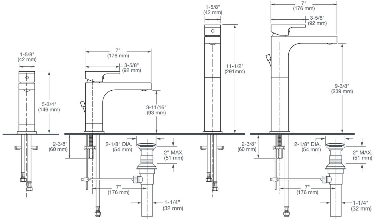
NOTE: MOUNTING HOLES ARE 1-3/8" D. (35 mm)
