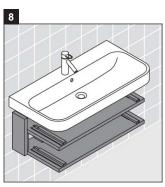
Slide the vanity under the washbasin. Tighten mounting nuts with a wrench until the washbasin is stable.
