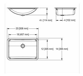
Single compartment undermount vanity basin. 18 gauge (1.2 mm), type 304 (CNS 18/10) stainless steel. Exposed surfaces are #4 satin finished. Undercoated to reduce condensation and resonance. Includes cutout template. Certified to ASME A112.19.3-2008 / CSA B45.4-08. Center back waste location, accepts 1 1/4" (32 mm) waste assembly (not included).
