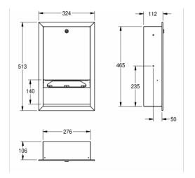
Paper towel dispenser for recessed mounting, stainless steel, surface satin finished, material thickness 22 gauge, folded front cover, cylinder lock with Franke standard key, loading capacity 500 - 800 pcs. of paper depending on convolution, including stainless steel screws and dowels.
