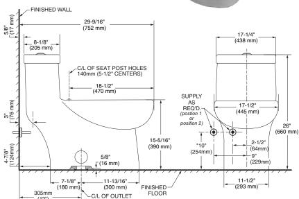
IMPORTANT: Water supply on the wall is required at 2-1/2" (64mm) or 9" (229mm) from centerline of the toilet (see rough-in). First suggested position is hidden behind the toilet. The geometry of the toilet gives space for this installation. The second suggested position is next to the toilet. Between these two positions, the space for the supply between wall and toilet is limited to 4-7/8" (124mm). In this case, check your supply and hose dimensions.
