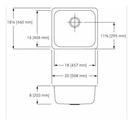
Single compartment undermount sink. 18 gauge (1.2 mm), type 316 (EN1.4401 17/12/2) stainless steel. Exposed surfaces are #4 satin finished. Undercoated to reduce condensation and resonance. Includes waste fitting, cutout template, and installation hardware. Certified to ASME A112.19.3-2008 / CSAB45.4-08.
